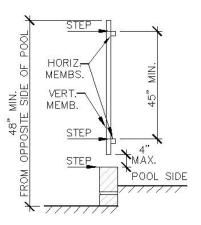
SCENARIO B IF VERT. MEMB. SPACING IS MORE THAN 13/4" BUT LESS THAN 4", PROVIDE 45" MIN. BETWEEN TOPS OF HORIZ. MEMBS.
