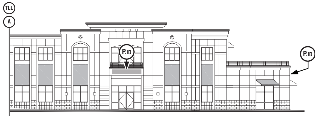
RESTAURANTS B / NORTH ELEVATION (PARKING LOT SIDE)
