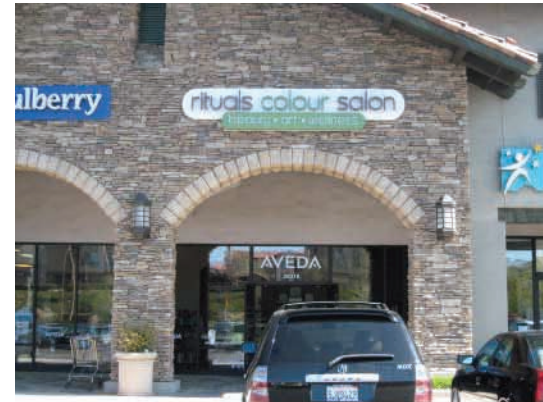
Fabricated back panel with reverse channel letters pin mounted off of face, large letters halo illuminate, lower letters are push thru acrylic
