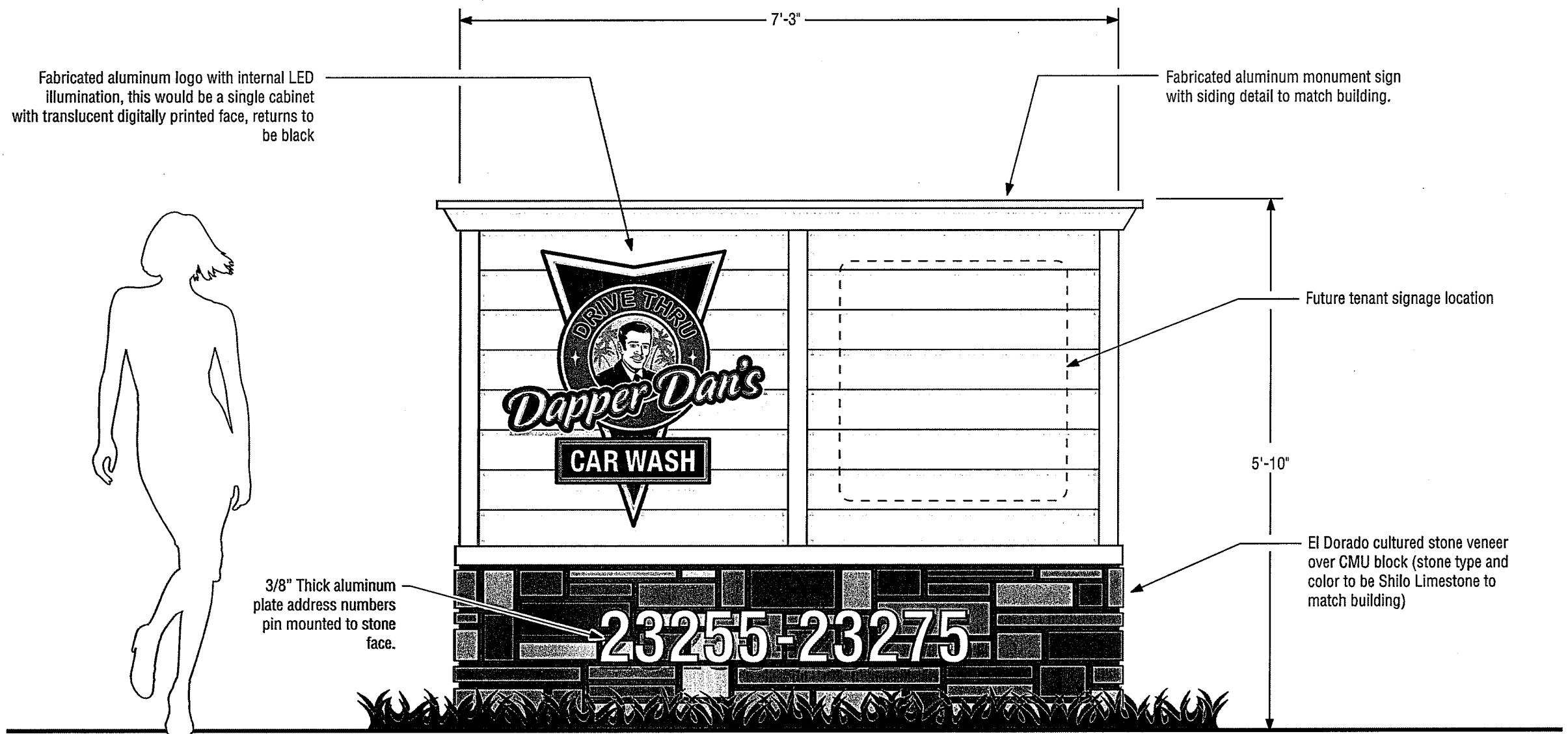
SIGN TYPE M2, M3 & M4 (MULTI-TENANT D/F MONUMENT SIGN) (sign area: 42.5 Sq. Ft.)
