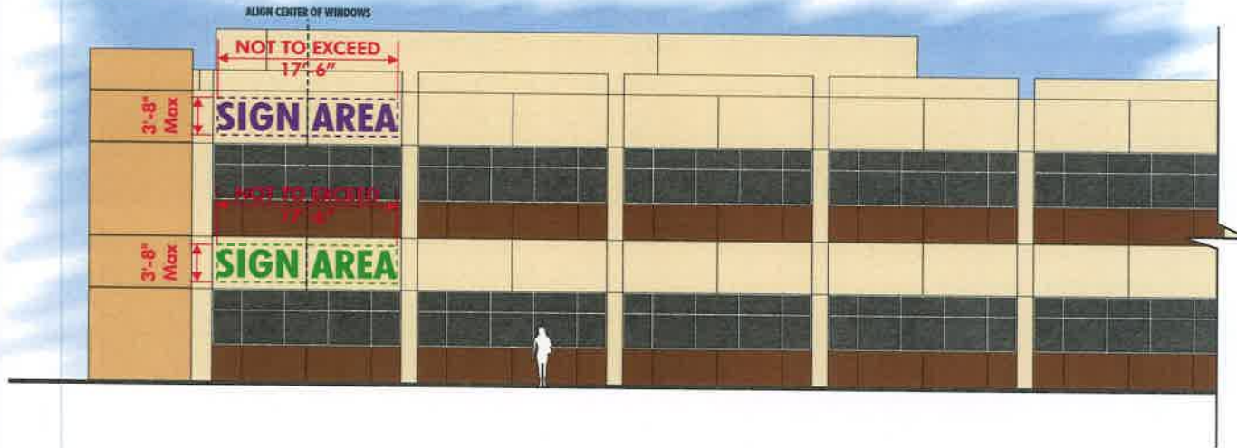
TS-2 North Elevation - Left Side Scale: 3/32" = 1' - 0"
