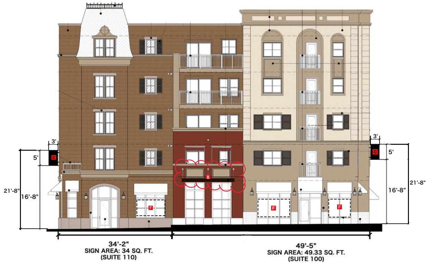
1 MAIN STREET EXTERIOR ELEVATION (WEST) - BUILDING A SCALE: 1/16" = 1'-0"
