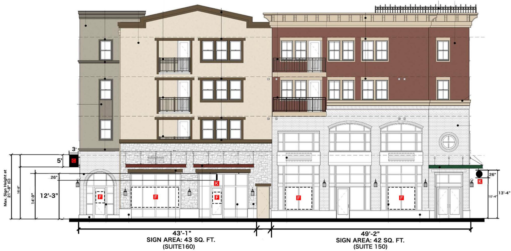
1 NORTH EXTERIOR PLAZA ELEVATION - BUILDING B SCALE: 1/16" = 1'-0"
