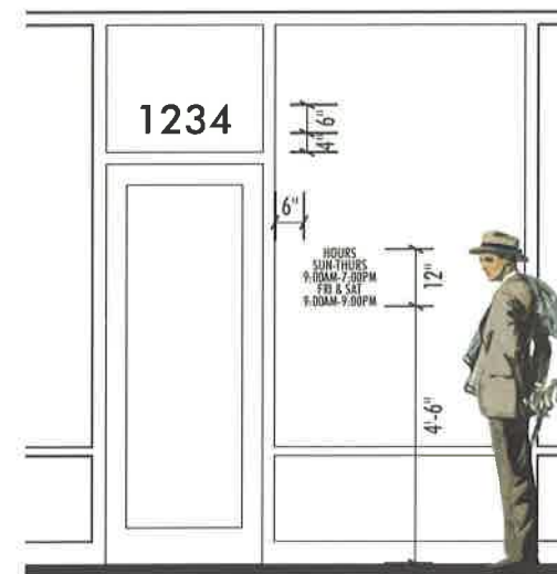
TYPICAL FRONT ENTRY ELEVATION
