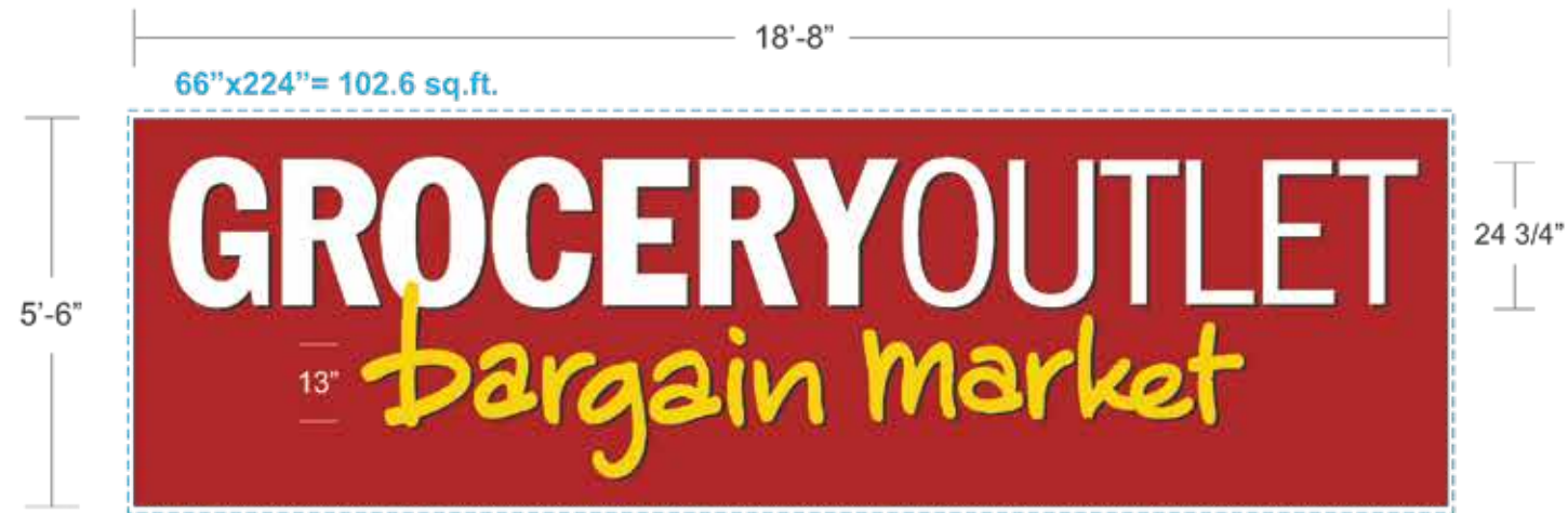
Sign C: Led Illum. P/C Sign on Alum. Bkgd (w/ behind the wall r/w) Scale 1/4"=1'-0"
