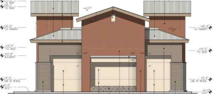
Building "C" South (side) Elevation: 1" = 20'-0"
