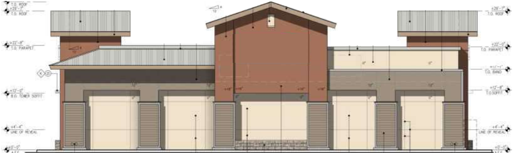
Building "C" East (back) Elevation: 1" = 20'-0"
