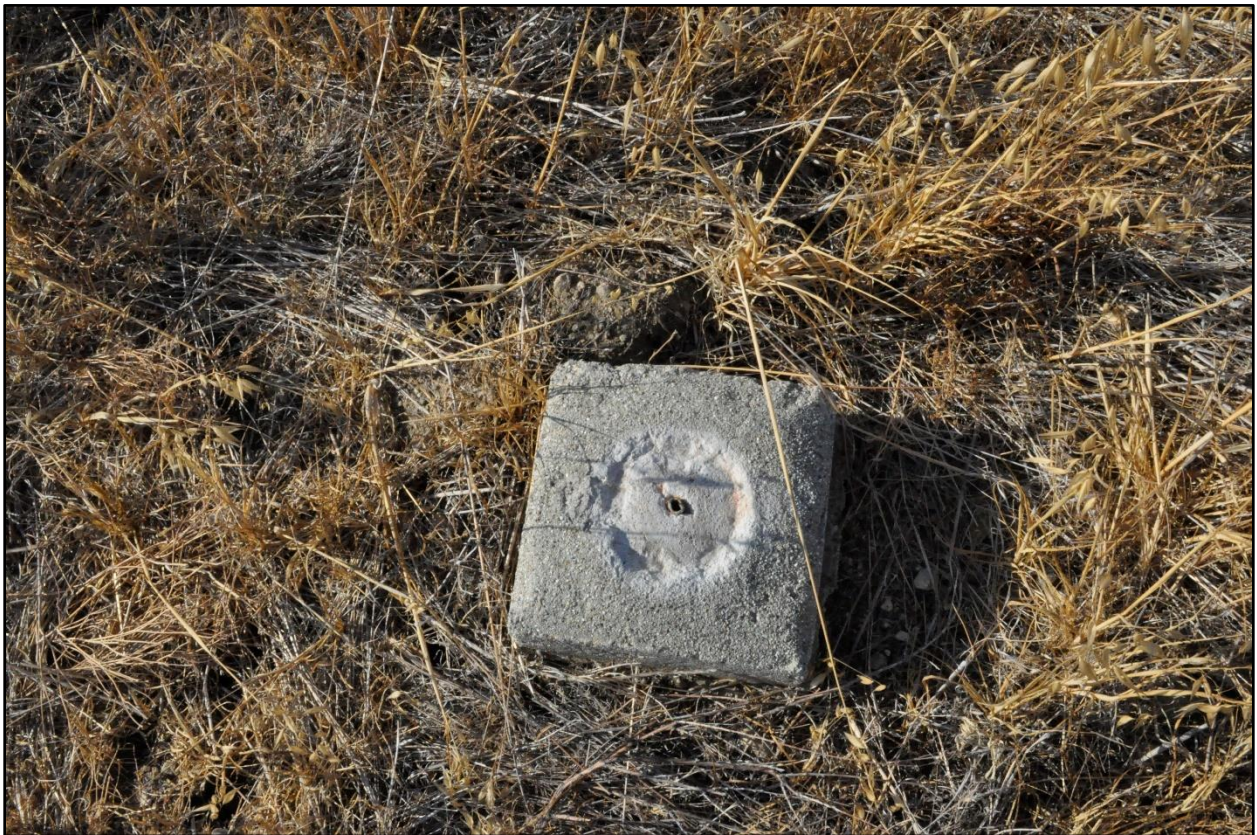
Figure 4. Top view of survey marker found atop the Project northern property line.
