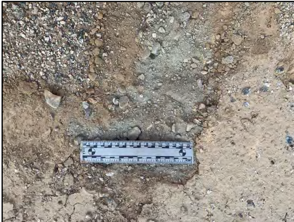
Figure 8. Lithology of unmapped Recent artificial fill and/or Holocene and late Pleistocene young alluvium, undivided (Qya). Plan view.
