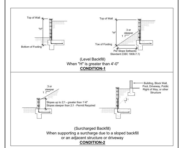
A permit is not required when retaining walls support less than 4 feet of level soil measured from the bottom of the footing to the top of the wall, unless supporting a surcharge.
