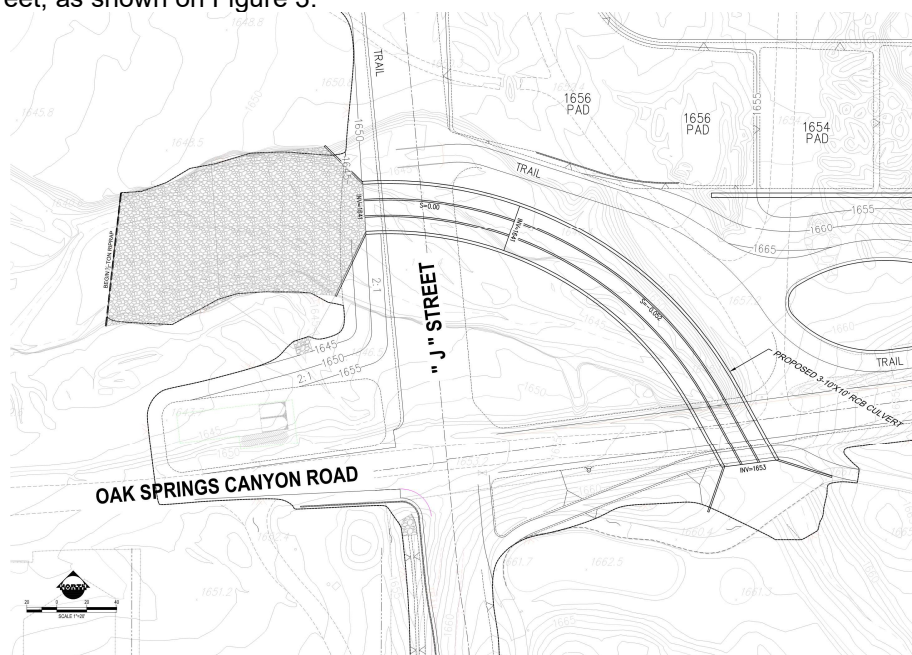
Figure 3: Revised Design at Oak Springs Canyon Road Culvert and Future J Street
